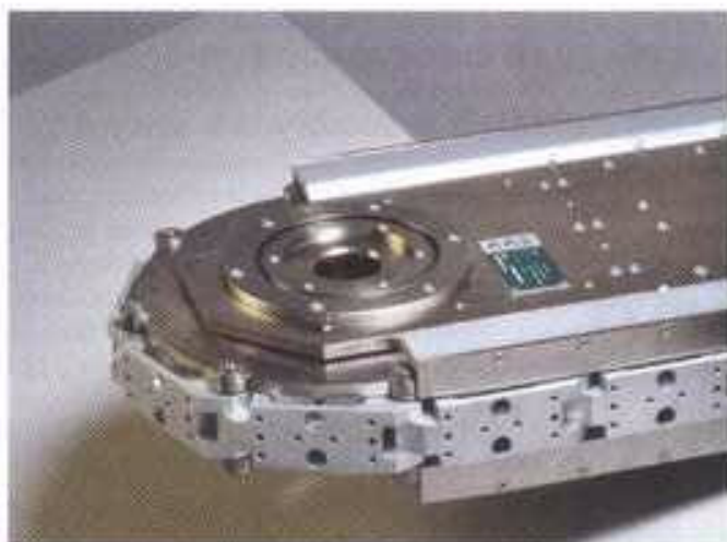
Fig. 2. The different product carriers are bolted to the chain links of the linear conveying system and can be positioned very exactly without locking
